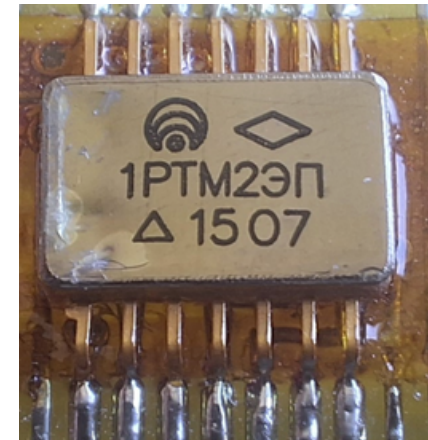
Dual CMOS D-type flip-flop with logic-level and clock inputs Manufacturing date: February 2015
